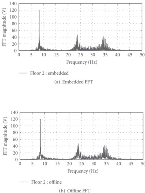
Figure 4. Comparison of FFT results. (a) Embedded using the wireless sensing unit. (b) Offline using MATLAB
