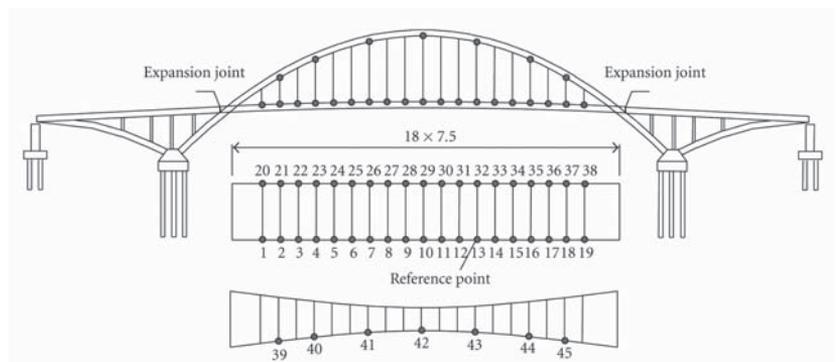
The uniaxial accelerometer has a sensitivity of 1 V/g with a resolution of  $10^{-6}$  g, while the triaxial one has values of 8 V/g and  $1.6 \times 10^{-7}$  g, respectively. For the data acquisition by the wireless sensing network,
