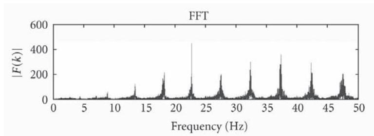
forces utilizing (4), which does not require all the peaks in the frequency spectrum, the first and the second vibration frequencies of the cable are not necessary in this study.
