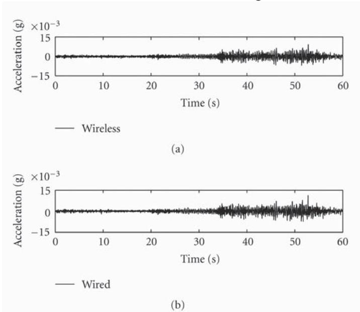
Figure 7. Vertical acceleration time history recorded by sensing node 2
