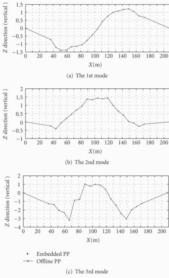
Figure 9. Comparison of mode shapes estimated by embedded and offline PP
