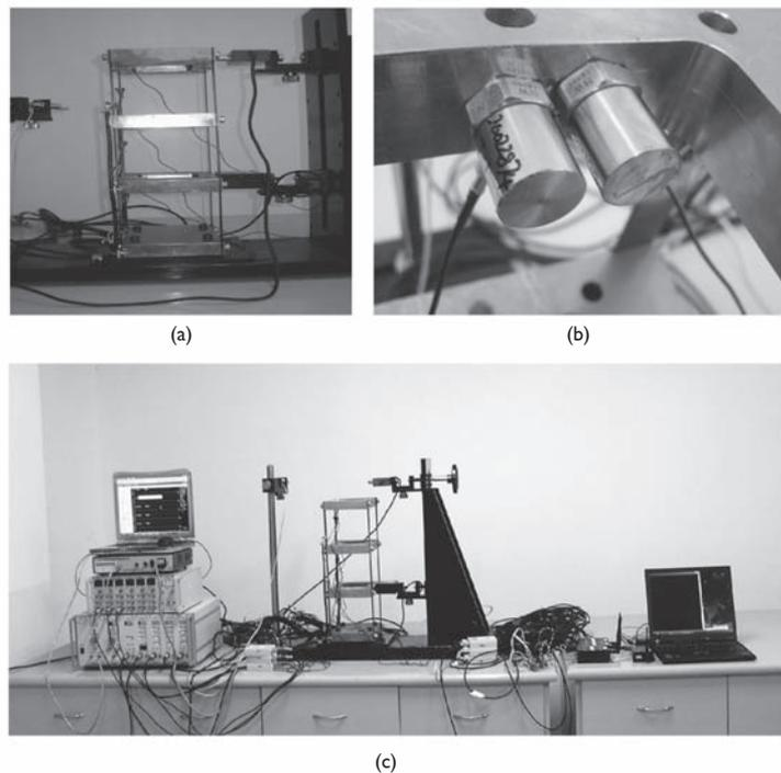
First, the time-history response data is transformed to the frequency domain via the embedded FFT algorithm. Embedded computing time of the 4096-point FFT by the microcontroller is around 16.5 seconds. Based upon the datasheets of the components in the wireless sensing unit (Wang et al., 2007; MaxStream Inc., 2005), during embedded computing, the micro controller together with
