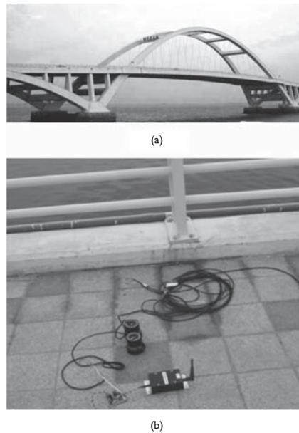
Due to the easy installation of wireless sensors in the field, 45 locations on the bridge deck and arch ribs are mounted with uniaxial or triaxial accelerometers, manufactured by Harbin Institute of Engineering Mechanics, to measure the corresponding vertical and transverse acceleration responses of the bridge under ambient excitation (Figure 6).
