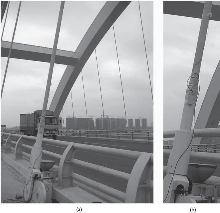
Figure 10. Accelerometer with wireless sensor on a hanger
