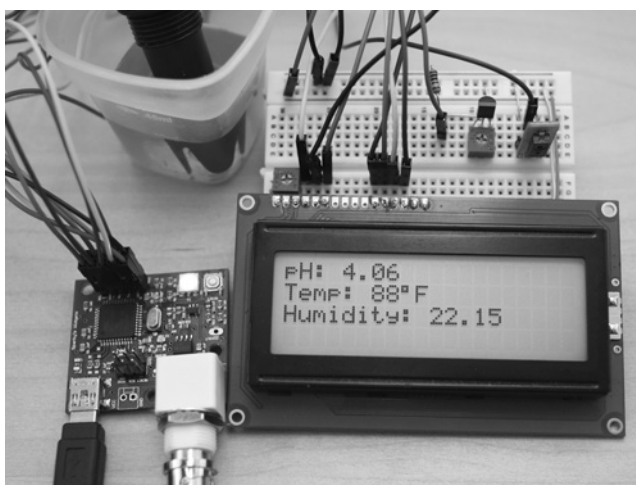
Figure 1. pH-meter realized with Arduino. The system also permit to measure temperature and humidity in a chemical solution
