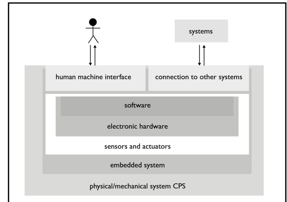
**Figure 1.** Interaction between humans and machines via Cyber-Physical- Systems
